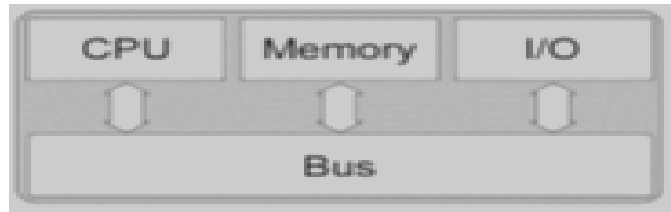
Figure.1 Three Main Components of a Microcontroller Source : Naga and Widiatmoko (2023)
