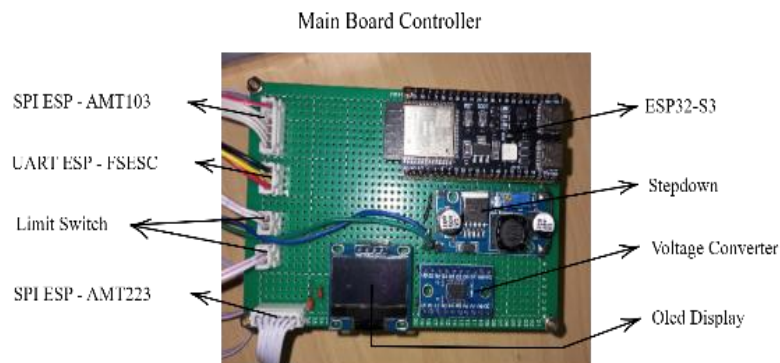
Figure 8. Main Board System of Cart Inverted Pendulum (Source : Author's Documentation, 2024)
